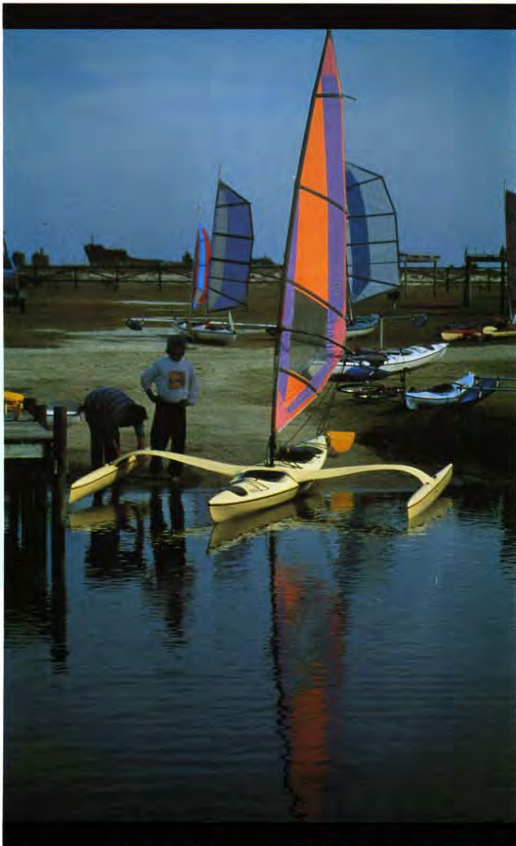
Available in 1993, Seascape/Tri-ka with wing and hard shell outriggers. This can be adapted with a windsurfing sail. Wing and outriggers designed by Rick Jones.
