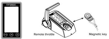
The remote throttle is equipped with a magnetic key with an off/off function. The motor only works if you place the magnetic key supplied on the proper groove on the remote throttle lever (see drawing). If the magnetic key is removed the motor stops. You can only start the motor again if you first replace the magnetic key and then move the remote throttle lever to the middle (neutral) position.
