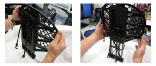
19. Attach the seat back pad to the seatback by hooking the webbing on bottom of seat back pad on notch at bottom of seat back as shown.
