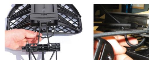
15. Pinch looped bungee to hold it in place under U-shaped slot in seat back spine, then flip riser over so it is right side up and positioned to be inserted into seat back spine.
